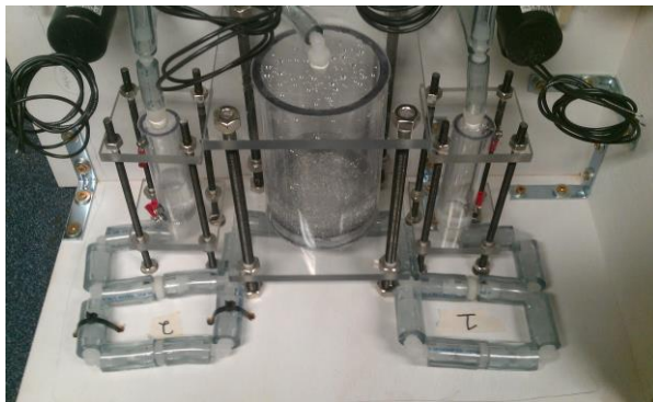
Fig 1: (left) Pistonless Pump Technology Demonstrator Mock-up Prototype (right) Current flight-ready design of the Pistonless Pump Technology Demonstrator Payload
